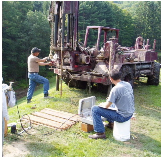
Figure 3 Dilatometer Test in progress at the top of the dam
